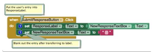
Figure 4-4. Setting the response to the user's entry
