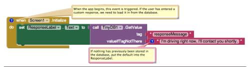
Figure 4-6. Loading the custom response from the database upon app initialization
