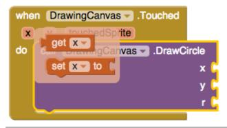
**Figure 2-9.** Mouse over an event parameter to drag out a get block for obtaining the value
