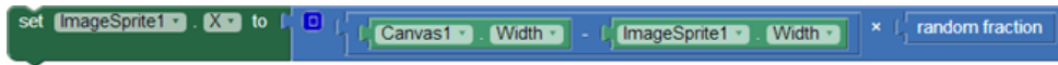
Figure 16-7. You can use Math blocks to build complex expressions like this one
