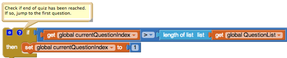
Figure 15-2. Using a comment on the if block to describe what it does in plain English
